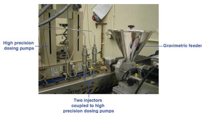
Figure 2 Dual-Injector Apparatus. [Color figure can be viewed in the online issue, which is available at www.interscience.wiley.com .]
